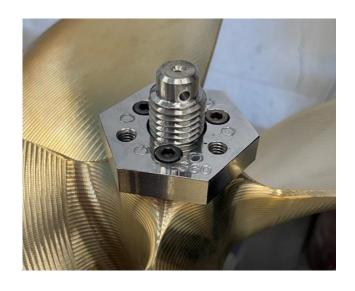
1) Place lower plate on back of hub and thread/tighten hex bolts to tapped holes of hub
