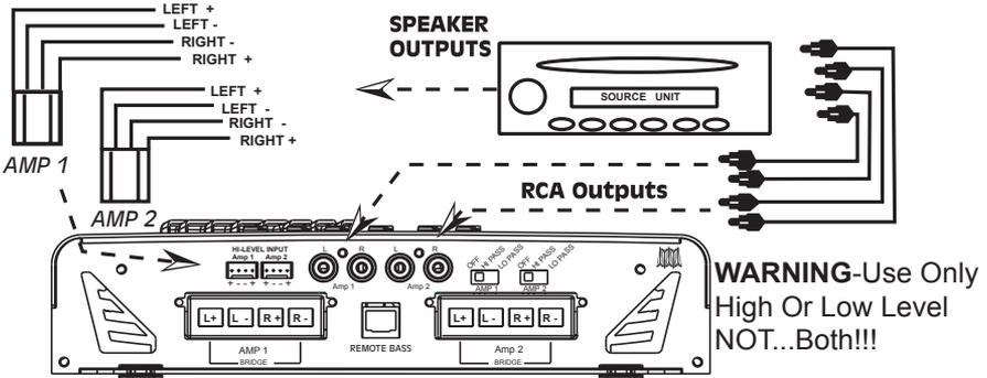
The use of twisted pair interconnects is recommended for all installations to minimize noise. When routing these cables through the automobile, try to keep them away from factory wiring harnesses and other power wiring. If you need to cross any of this wiring do so at a 90 degree angle to reduce the potential of noise problems.
