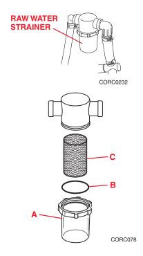
Clean debris from the bowl and screen and rinse parts in fresh water. Insert the screen, place the O-ring in the groove of the bowl and screw the bowl on hand tight. Be sure to open the water valve before starting the engine.
