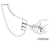
If the boat is pulling port **(A)**, rotate the foil to port **(B)** and tighten screws. If the boat is pulling starboard **(C)**, rotate the foil to starboard **(D)** and tighten screws. Always remember that movement of the trailing edge of the foil to one side will cause the steering to pull to the opposite side.
