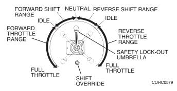
to REVERSE. Stay in NEUTRAL, or idle position until the boat has lost most of its headway before completing the shift to REVERSE or engine / transmission damage may
