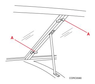
An open window can cause death or serious injury. Make sure both window locks are secure when vessel is in motion.
