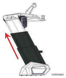
3. To start raising the tower, press and hold the "power" button. While holding the "power" button, press and hold the "up" button and the tower will begin to rise. (The "power" buttons are located near the back of the driver armrest.) Stop the tower at any time by releasing either of the buttons. The tower will support itself in this position until you command it to begin moving again.
