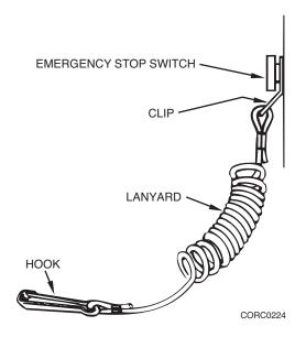
To attach a lanyard, connect the clip to the emergency stop switch and the hook to a strong piece of clothing on the operator, such as a belt loop.
