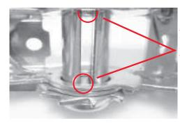
Apply a drop of lubricant as shown to both sides (top and bottom in this picture)
