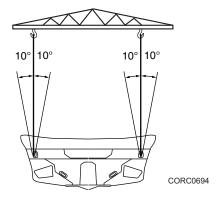
Drain the bilge and/or launch control system and/or aftermarket water bladder(s) to eliminate excess water before you lift the boat.
