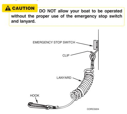
To attach a lanyard, connect the clip to the emergency stop switch and the hook to a strong piece of clothing on the operator, such as a belt loop.
