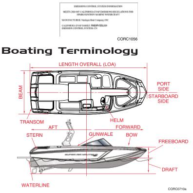
\* An easy way to remember PORT side from STARBOARD side is "PORT" and "LEFT" both have four letters.
