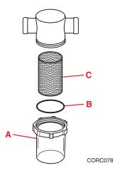
The raw water strainer bowl (A) remains full of water even after the rest of the engine cooling water system is drained. To properly winterize your boat, the strainer bowl must be removed and emptied. DO NOT lose the rubber O-ring (B) that seals the bowl to the cap. Clean screen (C) if required. If the water is not removed, the bowl can be damaged. A damaged strainer can cause overheating problems during the next season.
