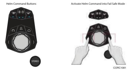
To enter Fail Safe Mode, press and hold the left and right arrow buttons together for 4 seconds. The "Start/Stop" button will be pulsing between white and off, and the lights on the Helm Command will begin to alternate red and white. Release the arrow buttons. You will now be able to enter your User Code by using the Helm Command buttons as numbers.
