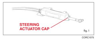
Remove the cap from the steering override cable guide tube (fig. 2) and thread the housing into the steering actuator.
