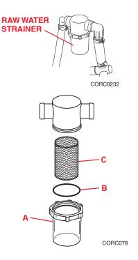
Clean debris from the bowl and screen and rinse parts in fresh water. Insert the screen, place the O-ring in the groove of the bowl and screw the bowl on hand tight. Be sure to open the water valve before starting the engine.
