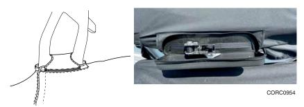
With the cover placed evenly around the boat and the buckles snapped closed at the tower base, unzip the ratchet strap pockets on the back of the mooring cover. Ratchet the strap, rotating from port ratchet to starboard ratchet, until the strap is tight.
