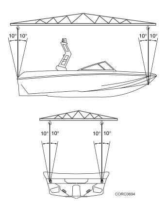
Drain the bilge and/or launch control system and/or aftermarket water bladder(s) to eliminate excess water before you lift the boat.
