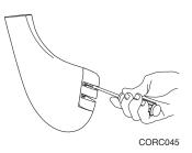
If the boat is pulling port **(A)**, rotate the foil to port **(B)** and tighten screws. If the boat is pulling starboard **(C)**, rotate the foil to starboard **(D)** and tighten screws. Always remember that movement of the trailing edge of the foil to one side will cause the steering to pull to the opposite side.
