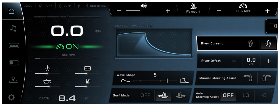
FIG. F8 - GPS RIVER MODE FOR BOATS EQUIPPED WITHOUT PADDLE WHEEL
