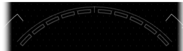
FIG. F6 - GREY COLORED GRAPHICS, STERN THRUSTER NOT IN USE AND AUTO STEERING ASSIST OFF
