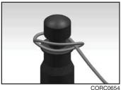
4. Tighten by pulling on the tail of the rope that leads to the skier.
