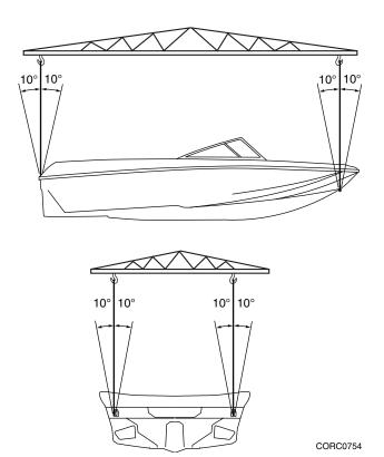
Drain the bilge and/or a launch control system and/or aftermarket water bladder(s) to eliminate excess water before you lift the boat.
