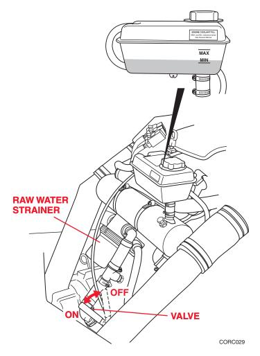
Some engines are equipped with a closed cooling system with a self-contained reservoir for engine coolant. Self-contained systems are equipped with a heat exchanger which uses raw water to cool the coolant. All raw water systems are equipped with a valve and strainer.
