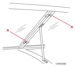
An open window can cause death or serious injury. Make sure both window locks are secure when vessel is in motion.
