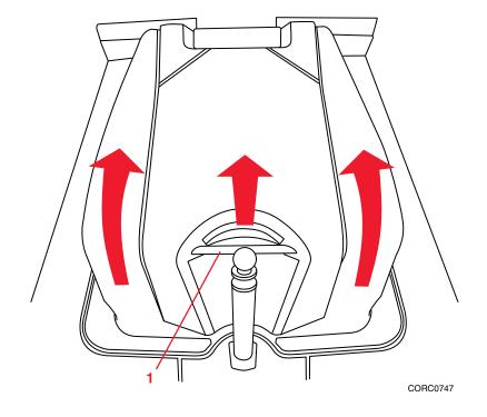
The engine box cover is heavy; be sure that all feet are clear of the box area when closing. Failure to do so may result in foot injury.
