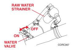
The raw water strainer bowl (A) remains full of water even after the rest of the engine cooling water system is drained. To properly winterize your boat, the strainer must be removed and emptied. DO NOT lose the rubber O-ring (B) that seals the bowl to the cap. Clean screen (C) if required. If the water is not removed, the bowl can be damaged. A damaged sea strainer can cause overheating problems during the next season.
