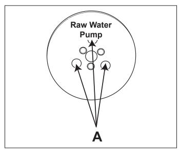
Raw Water Pump Impeller Bolt Locations "A"
