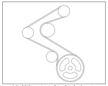
6.2L SC Supercharger Drive Belt Configuration
