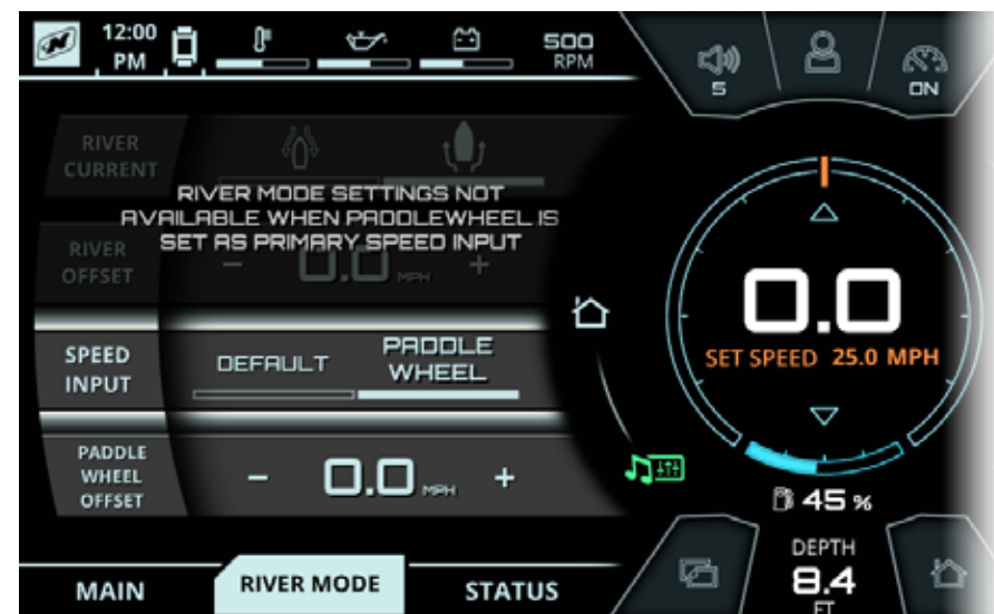
FIG. E3 - RIVER MODE TAB W/ PADDLE WHEEL SPEED INPUT
