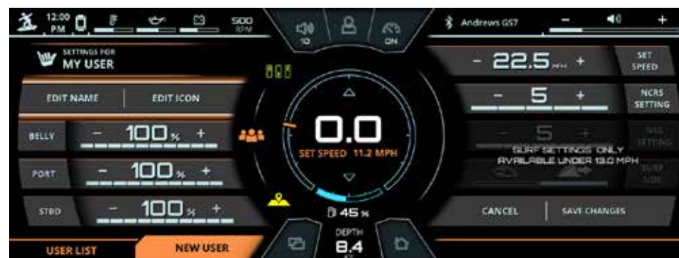
FIG. L4 - NEW USER TAB (EDIT USER SCREEN TO ADJUST SETTINGS)
