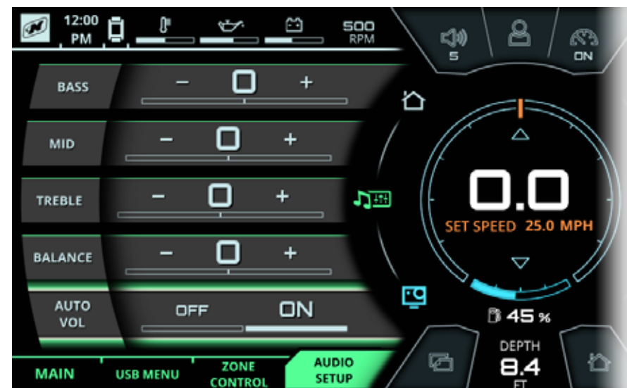
FIG. G6 - AUDIO SETUP TAB ON THE MEDIA MENU
