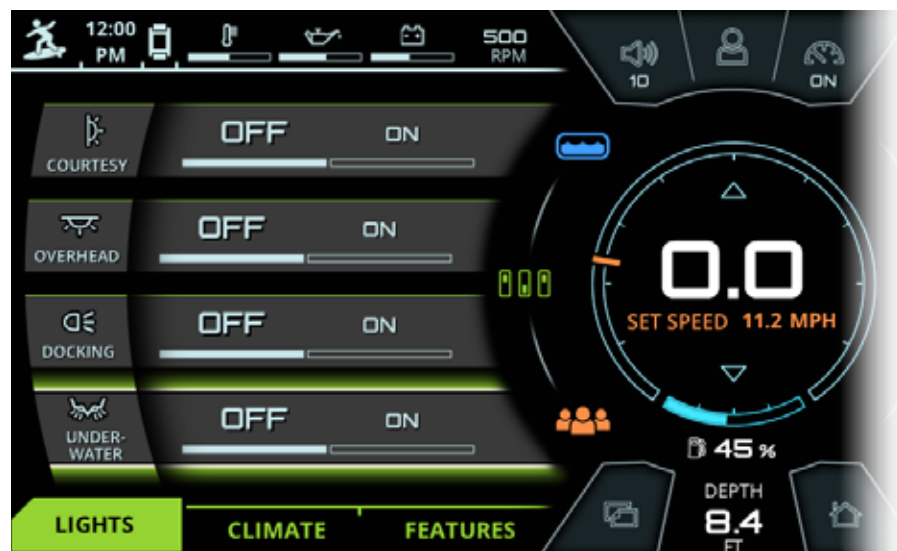
FIG. K1 - LIGHTS TAB* ON THE SWITCHING MENU
