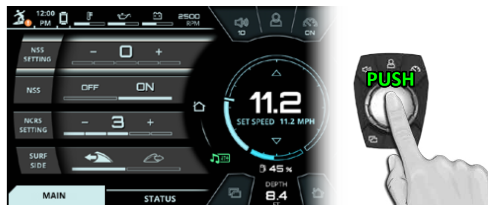
FIG. A6 - PUSHING DOWN TO DE-SELECT A SETTING (THE NSS SETTING IN THIS EXAMPLE)
