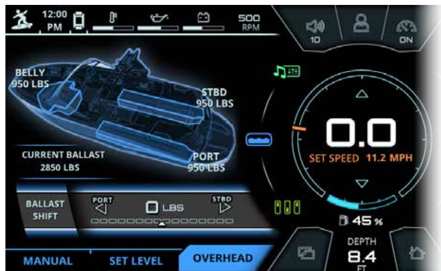
FIG. J3 - OVERHEAD TAB ON THE BALLAST MENU
