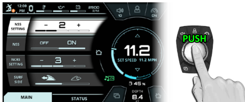
FIG. A4 - PUSHING DOWN TO SELECT A SETTING (THE NSS SETTING IN THIS EXAMPLE)
