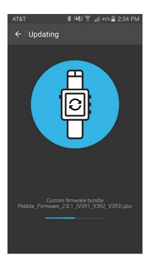
While the firmware is loading it is VERY important that the process is not interrupted. If the update process is interrupted this can result in the watch becoming unusable.
