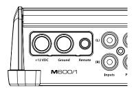
The M600/1's "+12 VDC" and "Ground" connections are designed to accept 4 AWG power wire. 4 AWG is the required wire size for this amplifier.
