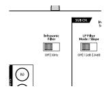
With ported enclosures and infinite baffle subwoofer systems, the use of the "Infrasonic Filter" is highly recommended to protect the speaker(s) from excessive excursion at inaudibly low frequencies.
