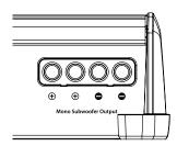
You will notice that there are two "+" positive connections and two "-" negative connections. This is to facilitate multiple subwoofer wiring. The two positive and two negative connections are connected in parallel inside the amplifier They are not stereo outputs. Connecting two subwoofers, each to one set of positive and negative terminals, will result in a parallel subwoofer connection. If only connecting one pair of subwoofer wires, it is not necessary to use both sets of connections.
