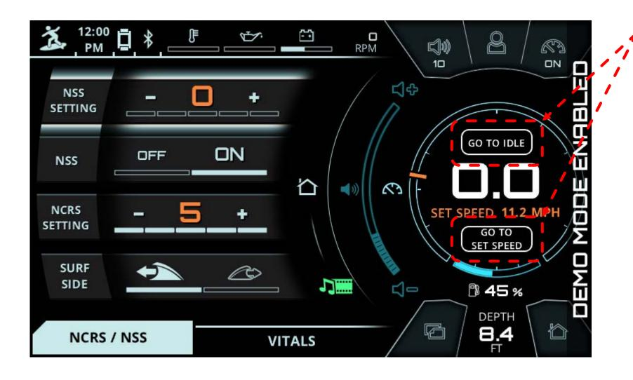
When "Speed Simulation" is enabled, two new buttons will show on any page that has a speedometer.
