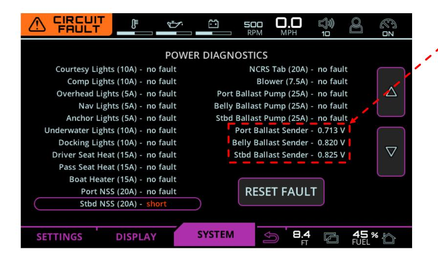
Displaying ballast sender voltages was added to 2016 V and G software.
