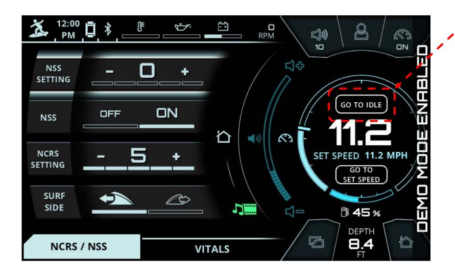
Pressing "Go To Idle" will simulate the boat decelerating down to zero. The NSS and NCRS plates will move and behave just as if the boat is actually slowing down.
