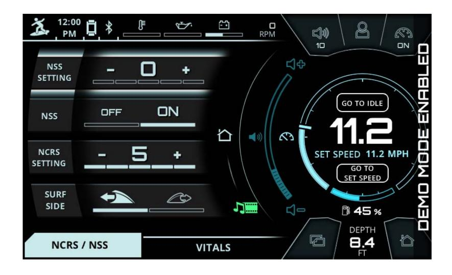
Once the set speed has been achieved, changing the settings on the LINC screen will also cause the NSS and NCRS plates to move like they would under normal boat operation.
