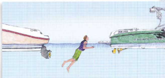
SAFETY. The prop on an inboard or v-drive boat is located under the boat ahead of the rudder, allowing safer boarding from the swim platform.
