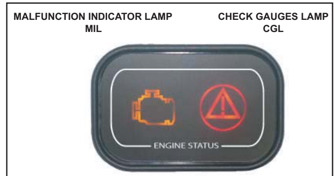
Figure 5-1A Typical Warning Lamp Cluster - CES Engines
