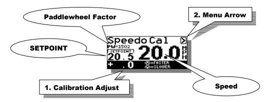
There is one speedometer calibration value for Wakeboard and Trick Modes: (If you calibrate in Trick Mode, Wakeboard is adjusted as well). If you calibrate, we recommend you do so at 20 mph.
