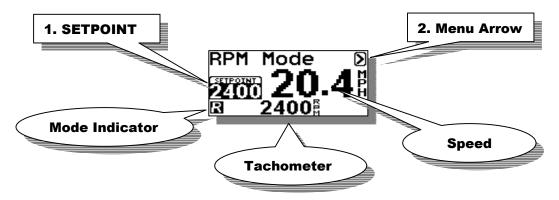
Operating in this mode is very similar to using the Wakeboard or Trick modes, except the system is now controlling to an RPM **SETPOINT**.
