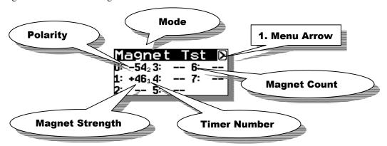
Timer Number- indicates the timer which has been triggered (labeled on Master Module "Timer 1" or "Timer 2").
