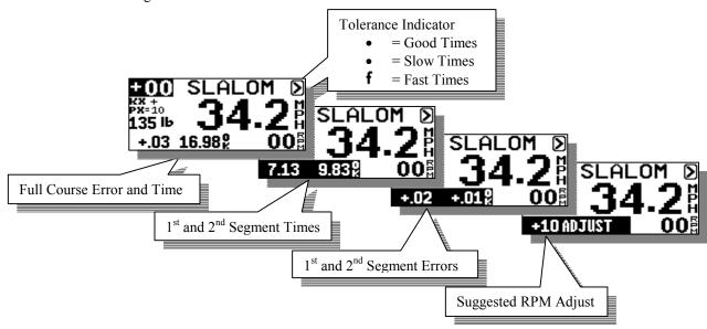
With the times highlighted on the screen you can press the **DOWN** key to view the All Buoy Timing information.
