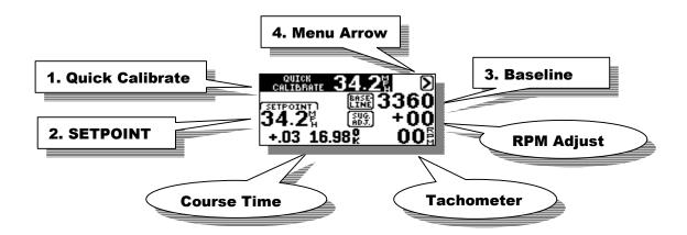
Your system must be calibrated for accuracy in a course. This is often called setting Baseline RPM Values / Calibration Screen. In slalom mode (without a skier) you must complete a timed slalom pass at each official speed you intend to use.
