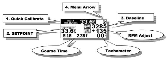
Press the **UP** key on the Quick Calibrate message to recalibrate the baseline based on the times recorded from the last pass. In this example it is suggesting your RPM Baseline should be increased by 135 rpm. When you perform a Quick Calibrate the suggested adjust of 135 will be added to the baseline and saved in memory. The system will also calibrate the digital speedometer if the times are with in the "OK" tolerance.
