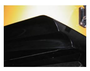
Curved chutes exhaust water cleanly without disturbance and without riding up the side.
