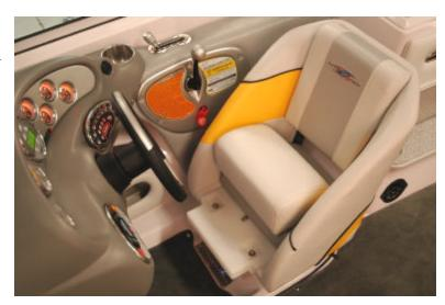
The driver's foot well is recessed to give even more leg room, plus it has snap in/out carpet and is self draining. Ballast gauges are readily in view by the right knee just above a nifty recessed storage bin. The driver's personal heater hose is located just ahead of the courtesy light under the master switch.
