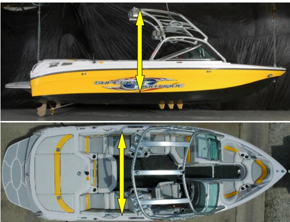
The new Flight Control Tower is powerful looking with a bold shape. Swivel board racks offer great storage and convenience. The tower clearance is 6'5" to the floor. Deafcon speakers take up nine inches. The beam inside the coaming pads is an amazing 78 inches making the 220 feel huge inside.
