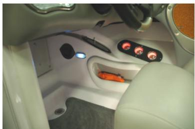
The 75 inch long locker is huge especially considering that there is 300 pounds of ballast capability in there as well. The Nautique logo on the water-proof locker pad adds another branded image. A larger latch is used to make accessing this area a breeze. The entire floor has snap in/out carpet over a diamond shape textured surface for easy cleaning and convenient use.
